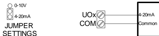
Figure 18: 4 to 20 mA Analog Output and Jumper Configuration
